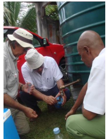
Figure 16 Chemical assessment; taking water samples on site
